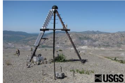
Tripod built in the 1980's serves as a modern GPS station at Studebaker Ridge, on the western flank of Mount St. Helens. View is to the north.
