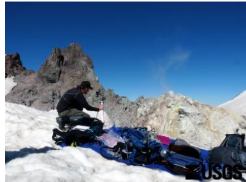
USGS geologist uses a UV spectrometer to detect gases from a fumarole at Crater Rock, Mount Hood, Oregon.
