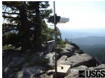
Seismic station at Three Sisters volcano in Central Oregon. Seismometer in box on the ground with data transmission antenna mounted on pole.
