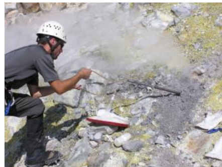
Gas sample being collected into a glass vacuum flask using a titanium tube inserted into a fumarole from Sherman Crater, Mount Baker, Washington.
