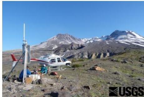
Scientists maintain an Acoustic Flow Monitor (AMF) at Mount St. Helens, Washington. It detects ground movement associated with lahars.
