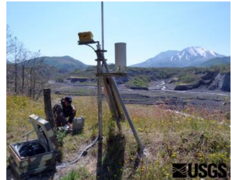
Acoustic Flow Monitoring station can detect ground vibrations of a passing lahar or debris flow and provide early warning to people downstream. Station near Mount St. Helens, Washington.
