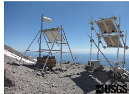
Seismic monitoring station SWFL—solar panels are used to recharge the batteries and keep the station running, Mount St. Helens.
