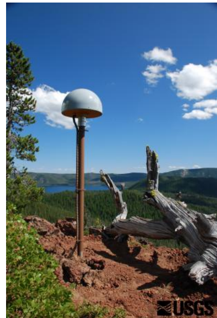
Global Positioning System receiver (called a GPS monument) at North Rim Station, a monitoring location at Newberry volcano, Oregon.
