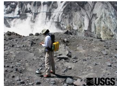
Gas sampling with a CO 2 Infrared Spectrometer at Mount St. Helens' September Lobe lava dome, Washington.
