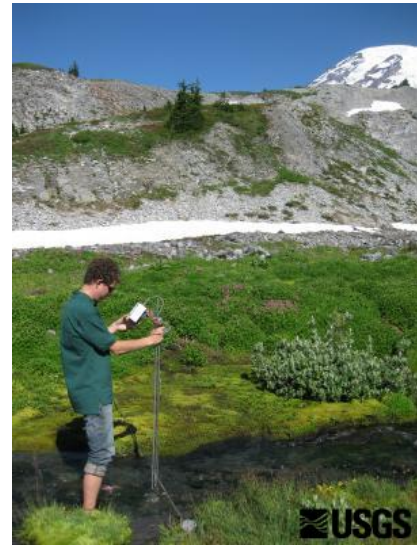
Streamflow measurement and water sampling at Paradise Creek are part of the regular measurements taken during hydrothermal monitoring campaigns at Mount Rainier, Washington.
