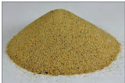
The mineral monazite is an important source of the REEs. Monazite, a REE-thorium-phosphate mineral, has been separated from some ancient and modern beach sands as a coproduct to the recovery of economic titanium (Ti) minerals. Photograph courtesy of www.geology.com .
