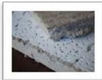
Perlite used in ceiling tiles dampens noise.
