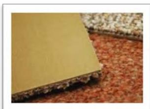
Aluminum trihydrate is used as a flame retardant filler in carpet backing.
